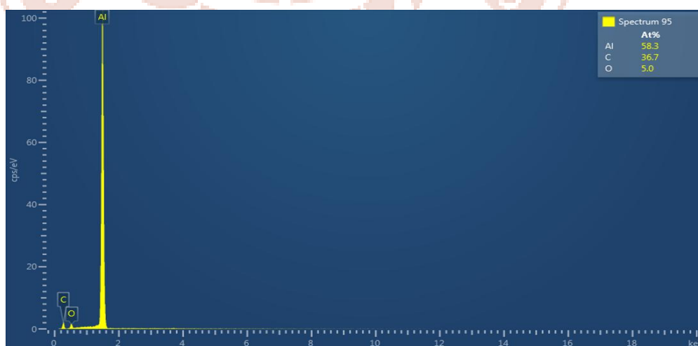
Fig. 8c: EDX images of the Aluminium surface after 24 h of immersion at 301 \pm K in 0.15 N NaOH in 2.0 gm/dL AILE.
